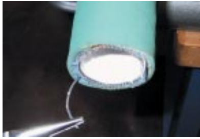
Pull out the helix wire end, if any.
