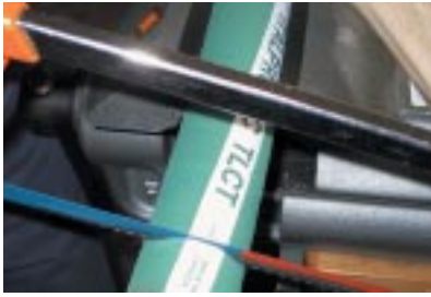
Cut the hose by means of a manual or automatic fine-toothed hacksaw.
