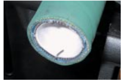
Bend it inside the hose, to guarantee conductivity, if required.
