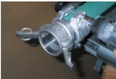
At the beginning use longer bolts to pull the two halves together.
